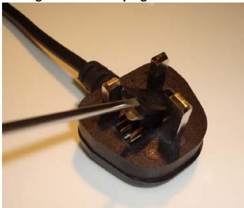
Figure 28: Mains plug fuse removal
